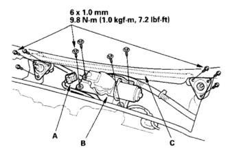
Remove the bolts, then remove windshield wiper linkage assembly (C). 5. Remove the three mounting bolts and nut from the wiper linkage (A) to remove the wiper motor (B).
