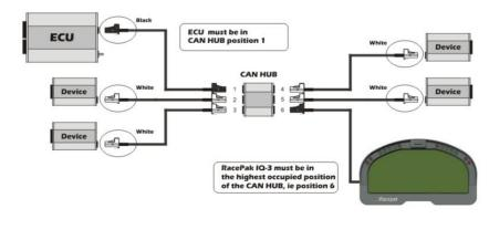
Figure 10 – Haltech ECU connected to 5 Auxiliary CAN based devices
