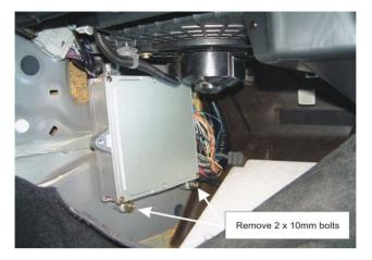
Figure 2 – Factory ECU removal
