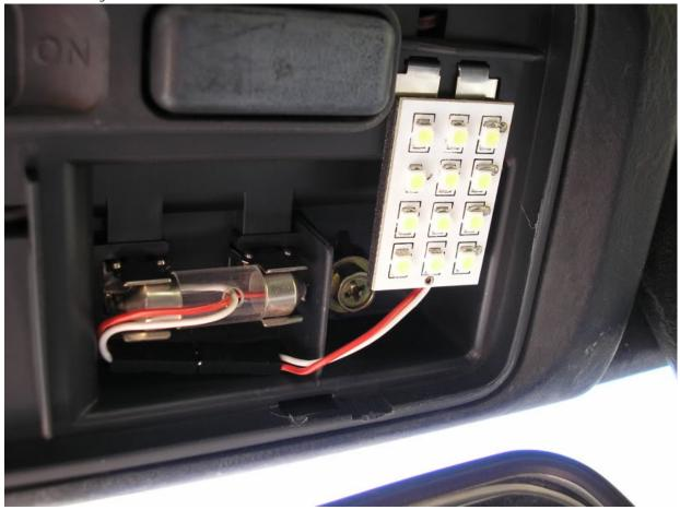
There are two small clips at the front of the light to pop off, then the light fixture comes down.
