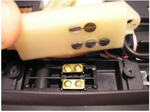
Remove the slide switch but BE CAREFUL, it's easy to lose the little ball bearing detent balls.
