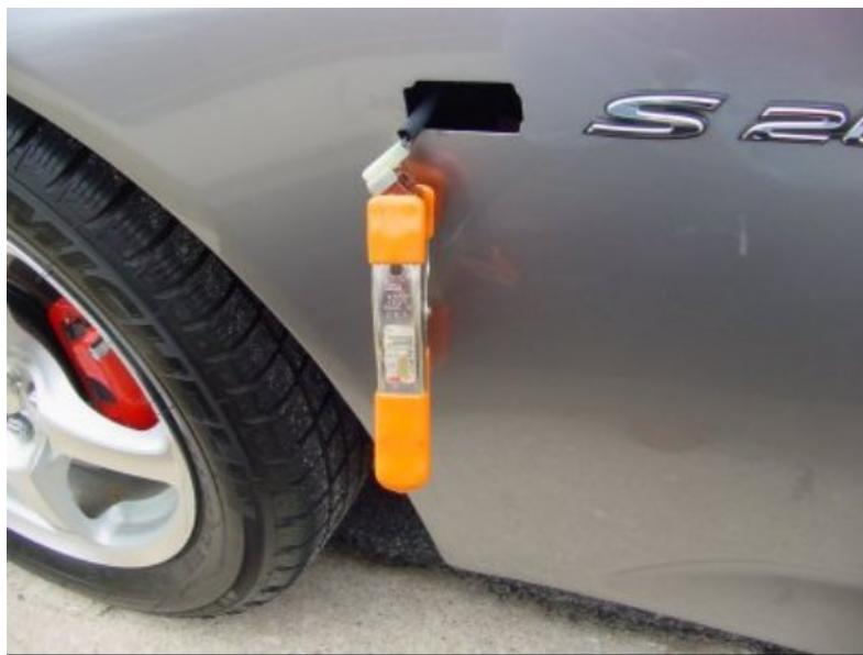
4. Plug the connector into the new marker, making sure the tab locks into place. Before installing the marker, operate the turn signal to be sure the marker is working.
