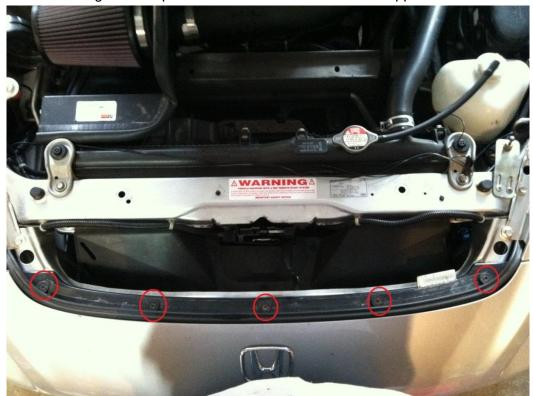
3. Using a 10mm socket, remove the bolt circled in red for the driver and passenger side (Note: Photo shows only driver side).
