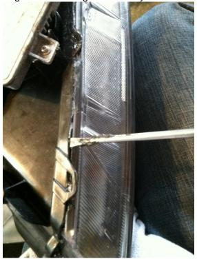
3. Once the edges have been lifted along the entire lens, reheat the entire edge of lens or re-bake the headlights one more time.
