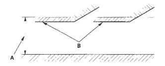
6. If necessary, adjust the headlights to local requirements by turning the vertical adjuster (A).
