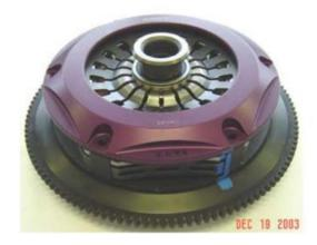
**NOTE:** The lower clutch disc is marked 'F/W SIDE' (Flywheel) and the upper clutch disc has 'T/M SIDE' (Transmission) on the plate. These clutch discs must be assembled with the logo facing towards the clutch cover.
