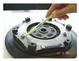
2. Place pressure plate on the spacer washers and release bearing in the centre of the clutch.
