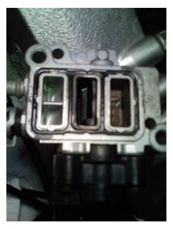
Use Carburetor Cleaner "liberally" to clean away the build up. Use an air hose to blow out the excess. This took some time for myself. I had a thick build up, so I repeated the application several times. WD-40 was tried first, and didn't do squat compared to the Carb Cleaner.
