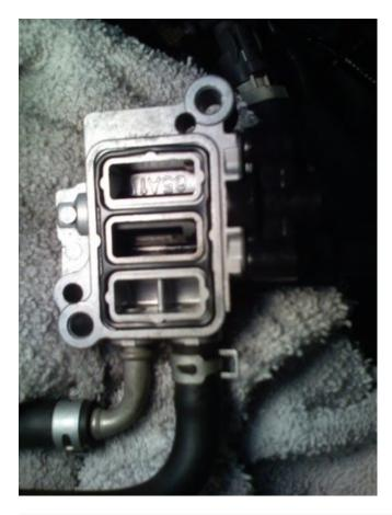
Rotate it back over and replace the two bolts. Be sure to start the bolts by hand and tighten them as much by hand as possible just to be safe.
