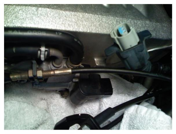
Push back the rubber boot off the plug on the right side of the IAC, and unplug it. You can see where to press in the pic.
