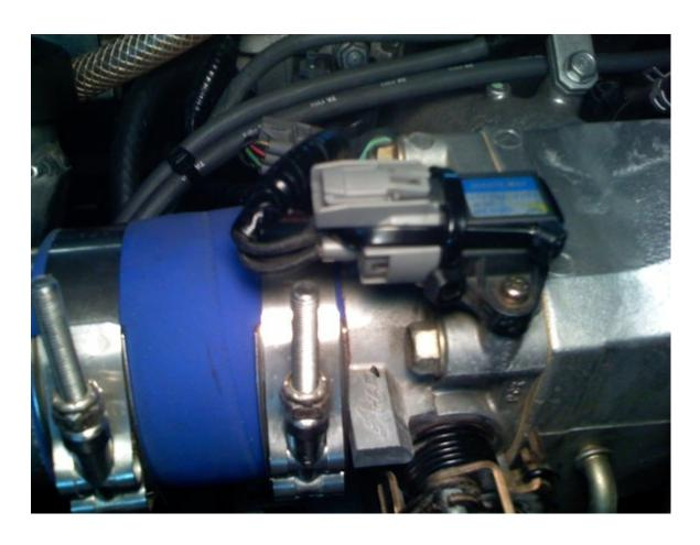
I also haven't had the MAP sensor zip tie fix from Honda so I just did a MAP WACK - unplugged and cleaned the plug (not the sensor) with Honda Brake Cleaner, allowed it to dry - replugged it and applied two zip ties to hold it tight.
