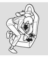
5. After confirming that the belt is locked, grab the shoulder part of the belt near the buckle, and pull up to remove any slack from the lap part of the belt. Remember, if the lap part of the belt is not tight, the child seat will not be secure.
