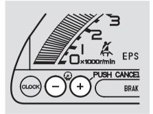
The buttons in the lower left corner of the instrument panel adjust the brightness of the display in five steps. Push the + or - button five times to see the full range.
