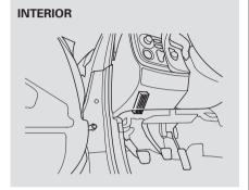
The interior fuse box is underneath the dashboard on the driver's side.
