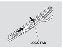
2. Disconnect the blade assembly from the wiper arm by pushing in the lock tab. Hold the lock tab in while you push the blade assembly toward the base of the arm.
