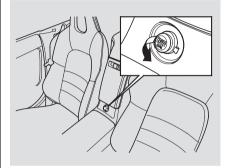
This socket is intended to supply power for 12 volt DC accessories that are rated 120 watts or less (10 amps).
