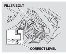
Check the fluid level with the differential at normal operating temperature and the vehicle sitting on level ground. Remove the differential fluid filler bolt and washer, and carefully feel inside the bolt hole with your finger. The fluid level should be up to the edge of the bolt hole. If it is not, slowly add fluid until it starts to run out of the hole. Use an SAE 90 viscosity hypoid gear oil, API service classified GL5 or GL6 only.
