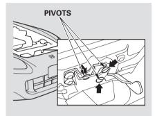
Clean the hood latch assembly with a mild cleaner, then lubricate it with a multipurpose grease. Lubricate all the moving parts (as shown), including the pivot. Follow the time and distance recommendations in the Maintenance Schedule. If you are not sure how to clean and grease the latch, contact your Honda dealer. Check the brake fluid level in the reservoirs monthly.
