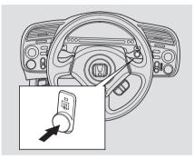
The rear window defogger will clear fog, frost, and thin ice from the window. Push the defogger button to turn it on and off. The indicator in the button comes on to show the defogger is on. If you do not turn it off, the defogger will shut itself off after about 15 minutes. It also shuts off when you turn off the ignition. You have to turn it on again when you restart the vehicle. Do not push the defogger button when the convertible top is folded.
