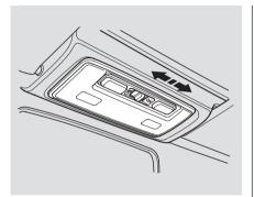
The interior light has a threeposition switch. In the OFF position, the light does not come on. In the center position, the interior light comes on when you open either door. In the ON position, the interior light stays on continuously. If the three-position switch is in the center position, the interior light will come on when you remove the key from the ignition switch.
