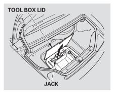
3. Open the trunk. Lift up the tool box lid, and take the jack, wheel wrench, and extension out of the tool box.
