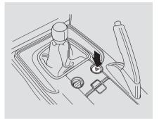
Push the red button next to the parking brake to turn on the hazard warning lights (four-way flashers). This causes all four outside turn signals and both indicators in the instrument panel to flash. Use the hazard warning lights if you need to park in a dangerous area near heavy traffic, or if your vehicle is disabled.
