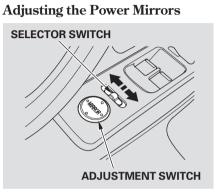
1. Move the selector switch to L (driver's side) or R (passenger's side).
