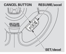
3. Press and release the SET/decel button on the steering wheel. The CRUISE CONTROL indicator on the instrument panel comes on to show the system is now activated.
