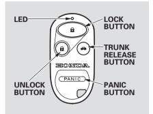
**LOCK** — Press this button to lock both doors. Some exterior lights will flash. When you push LOCK twice within 5 seconds, you will hear a beep to verify that the doors are locked.
