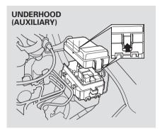
**Checking and Replacing Fuses** If something electrical in your vehicle stops working, check for a blown fuse first. Determine from the chart on pages 172 and 173 ,or the diagram on the fuse box lid, which fuses control that device. Check those fuses first, but check all the fuses before deciding that a blown fuse is the cause. Replace any blown fuses, and check if the device works.
