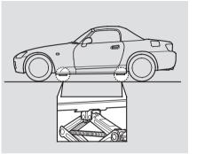
7. Locate the jacking point nearest the tire you need to change. It is pointed to by an arrow molded into the underside of the body. Place the jack under the jacking point. Turn the end bracket clockwise until the top of the jack contacts the jacking point. Make sure the center of the jacking point tab is resting in the jack notch.
