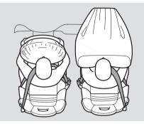
Your vehicle has a Supplemental Restraint System (SRS) with frontal airbags to help protect the heads and chests of the driver and a passenger during a moderate to severe frontal collision (see page 18 for more information on how your airbags work). The most important things you need to know about your airbags are:
