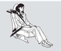
For added protection, the seat belts are equipped with automatic seat belt tensioners. When activated, the tensioners immediately tighten the belts to help hold the driver and the passenger in place. The tensioners are designed to activate primarily in frontal collisions, and they should activate in any collision severe enough to cause airbag inflation.
