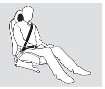
If necessary, pull up on the belt again to remove any slack, then check that the belt rests across the center of your chest and over your shoulder. This spreads the forces of a crash over the strongest bones in your upper body. *Never place the shoulder portion of a lap/shoulder belt under your arm or behind your back.* This could cause very serious injuries in a crash.
