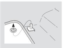
The driver's floor mat that came with your vehicle hooks over the floor mat anchor. This keeps the floor mat from sliding forward and possibly interfering with the pedals.
