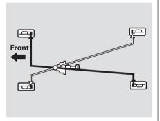
The hydraulic system that operates the brakes has two separate circuits. Each circuit works diagonally across the vehicle (the left-front brake is connected with the right-rear brake, etc.). If one circuit should develop a problem, you will still have braking at two wheels.
