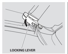
4. With the latches released, push the locking levers up until they latch.
