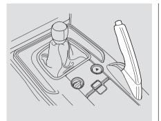
To apply the parking brake, pull the lever up fully. To release it, pull up slightly, push the button, and lower the lever. The parking brake indicator on the instrument panel should go out when the parking brake is fully released (see page 40). If you try to drive the vehicle without releasing the parking brake, the ABS indicator may come on, and the ABS may not work properly. **NOTICE:** Driving the vehicle with the parking brake applied can damage the rear brakes and axles.
