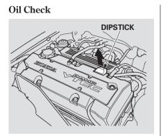
Wait a few minutes after turning the engine off before you check the oil.
