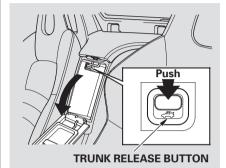
To open the trunk, press the trunk release button in the lower console compartment. To protect items in the trunk when you need to give the key to someone else, lock the lower console compartment with the master key, and give the other person the valet key.
