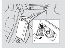
The area between the seat has two compartments. Open the lower compartment by squeezing the handle. Close it with a firm push. You can lock or unlock the lower compartment with the master key.
