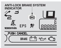
If the ABS indicator comes on, the anti-lock function of the braking system has shut down. The brakes still work like a conventional system, but without anti-lock. You should have the dealer inspect your vehicle as soon as possible. *Important Safety Reminders* ABS does not reduce the time or distance it takes to stop the vehicle. It only helps with the steering control during braking.
