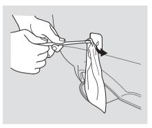
For very short distances, such as freeing the vehicle, you can use the detachable towing hook that mounts on the anchors in the front and rear bumpers.
