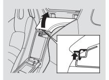
The lever to open the upper compartment is inside the lower compartment. Push up the lever, and lift the lid. To close, lower the lid, and push it down until it latches.
