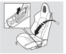
To change the seat-back angle, pull up on the lever on the outside of the seat bottom. You vehicle's windows are electrically-powered. Turn the ignition switch to ON (II) to raise or lower either window.
