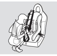
4. After the belt has retracted, tug on it. If the belt is locked, you will not be able to pull it out. If you can pull the belt out, it is not locked, and you will need to repeat these steps.
