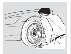
11.Put on the spare tire. Put the wheel nuts back on finger-tight, then tighten them in a crisscross pattern with the wheel wrench until the wheel is firmly against the hub. Do not try to tighten them fully.
