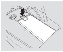
Open the beverage holder by pushing on the tab. The lid will slide open.
