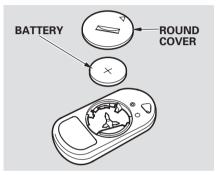
If it takes several pushes on the button to lock or unlock the doors, replace the battery as soon as possible. Battery type: CR2025 To replace the battery, remove the round cover on the back of the transmitter by turning it counterclockwise with a coin. Insert a new battery with the + side facing up. Align the  $\bigtriangledown$  mark on the cover with the  $\bigcirc$  mark on the transmitter. Set the cover in place, and turn it clockwise.
