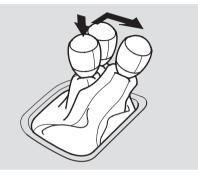
The 6-speed manual transmission has a lockout so you cannot accidentally shift from Fifth to Reverse instead of Sixth.
