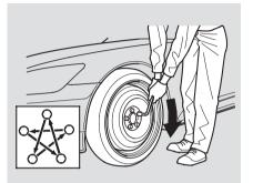
13. Tighten the wheel nuts securely in a crisscross pattern. Have the wheel nut torque checked at the nearest automotive service facility. Tighten the wheel nuts to: 80 lbf·ft (108 N·m , 11 kgf·m)
