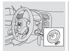
The ignition switch has three positions: LOCK (0), ACCESSORY (I), and ON (II).
