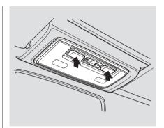
In addition, when the three position switch is in the center position with both doors closed, the two bulbs in the interior light can be turned on separately by the pushbutton switches next to them. Push the switch to turn the light on or off.
