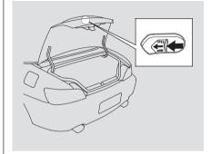
As a safety feature, your vehicle has a release lever on the trunk latch so the trunk can be opened from inside. To open the trunk, push the release lever to the left.
