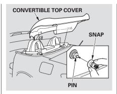
2. Pull the buttons on the snaps, place them over the pins on the back of the roll bar, then release the buttons. If you do not pull the snap button before placing it on the pin, you could break the snap.
