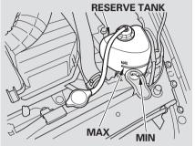
Look at the coolant level in the radiator reserve tank. Make sure it is between the MAX and MIN lines. If it is below the MIN line, see **Adding Engine Coolant** on page 132 for information on adding the proper coolant.
