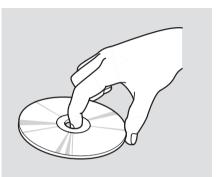
Handle a CD by its edges; never touch either surface. Do not place stabilizer rings or labels on the CD. These, along with contamination from fingerprints, liquids, and felt-tip pens, can cause the CD to not play properly, or possibly jam in the drive. If you see an error message in the display while playing a CD, find the cause in the chart to the right. If you cannot clear the error message, take your vehicle to a Honda dealer.
