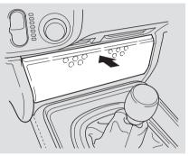
To open the audio panel, push on the top center, and let the panel swing down. To close, pivot the panel up, and push on it until it latches. The heating and air conditioning systems in your Honda provide a comfortable driving environment in all weather conditions.
