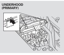
There are two under-hood fuse boxes in the engine compartment.
