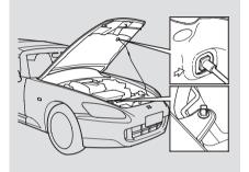
Lift it up slightly to remove the support rod from the hole. Put the support rod back into its holding clip. Lower the hood to about a foot (30 cm) above the fender, then let it drop. Make sure it is securely latched.
