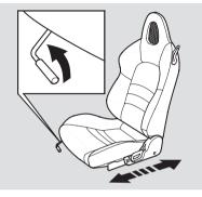
To adjust the seat forward and backward, pull up on the lever under the seat cushion's front edge. Then try to move the seat to make sure it is locked in position.
