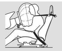
If you ever have a moderate to severe frontal collision, sensors will detect the vehicle's rapid deceleration. If the rate of deceleration is high enough, the control unit will instantly inflate the drivers and passenger's airbags. During a frontal crash, your seat belt restrains your lower body and torso, and the airbag helps protect your head and chest.
