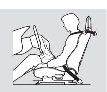
After inflating, the airbags will immediately deflate, so they won't interfere with the driver's visibility, or the ability to steer or operate other controls.
