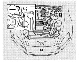
4. Connect the second jumper cable to the negative (—) terminal on the booster battery. Connect the other end to the metal projection near the intake manifold as shown in the illustration. Do not connect this jumper cable to any other part of the engine.
