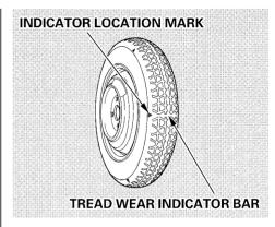
The compact spare tire has a shorter tread life than a regular tire. Replace it when you can see the tread wear indicator bars. The replacement should be the same size and design tire, mounted on the same wheel. The compact spare tire is not designed to be mounted on a regular wheel, and the compact wheel is not designed for mounting a regular tire.
