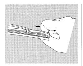
3. Remove the blade from its holder by grasping the tabbed end of the blade. Pull firmly until the tabs come out of the holder.
