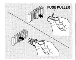
4. Check the smaller fuses by pulling out the fuse with the fuse puller provided in the interior fuse box.
