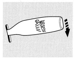
This lever controls the windshield wipers and washers. It has five positions;
