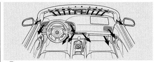
Air flow is divided between the floor vents, the defroster vents at the base of the windshield and the vents on both sides of the instrument panel.
