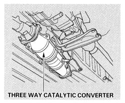
A defective three way catalytic converter contributes to air pollution, and can impair your engine's performance. Follow these guidelines to protect your car's three way catalytic converter.
