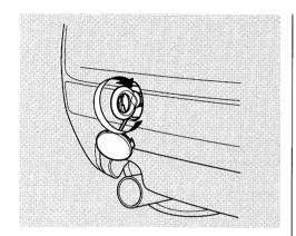
4. Screw the towing hook into the extension and tighten it securely by hand.
