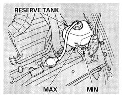
If the coolant level in the reserve tank is at or below the MIN line, add coolant to bring it up to the MAX line. Inspect the cooling system for leaks. This coolant should always be a mixture of 50 percent antifreeze and 50 percent water. Never add straight antifreeze or plain water.
