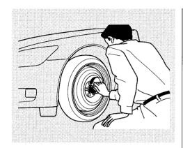
11. Put on the spare tire. Put the wheel nuts back on finger-tight, then tighten them in a crisscross pattern with the wheel wrench until the wheel is firmly against the hub. Do not try to tighten them fully.
