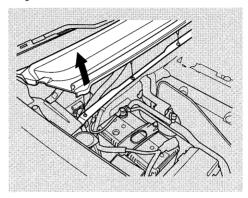
The air conditioning filter is located in the engine compartment on the passenger's side near the base of the windshield.
