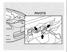
Clean the hood latch assembly with a mild cleaner, then lubricate it with a multipurpose grease. Lubricate all the moving parts, including the pivot. Follow the time and distance recommendations in the Maintenance Schedule. If you are not sure how to clean and grease the latch, contact your Honda dealer.
