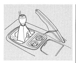
The manual transmission is synchronized in all forward gears for smooth operation. It has a lockout so you cannot shift directly from Fifth to Reverse instead of sixth (see page 134). When shifting up or down, make sure you push the clutch pedal down all the way, shift to the next gear, and let the pedal up gradually. When you are not shifting, do not rest your foot on the clutch pedal. This can cause your clutch to wear out faster.
