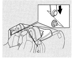
3. Hook the fastener string to the pin on each side wall of the passenger compartment.
