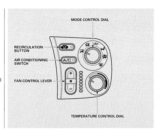
These settings direct all the air flow to the defroster vents at the base of the windshield and the side window defroster vents. The air flow will get warmer and clear the windows faster as the engine warms up. You can close the side vents with the dial beside each vent. This will send more warm air to the windshield defroster vents.
