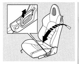
To change the angle of the seat-back, pull up on the lever on the outside of the seat bottom. Move the seat-back to the desired position and release the lever. Let the seat-back latch in the new position.
