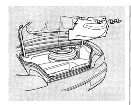
4. Remove the three clips holding the spare tire cover by pulling straight up on the rings. Remove the spare tire cover.
