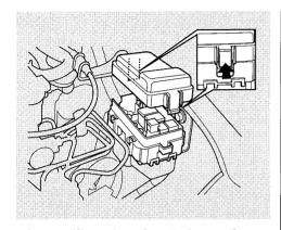
The auxiliary fuse box is located on the driver's side near the brake fluid reservoir. To open it, push the tab on each side and remove the lid.
