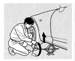
8. Use the extension and wheel wrench as shown to raise the car until the flat tire is off the ground.
