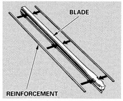
4. Examine the new wiper blades. If they have no plastic or metal reinforcement along the back edge, remove the metal reinforcement strips from the old wiper blade and install them in the slots along the edge of the new blade.
