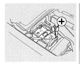
3. Connect one jumper cable to the positive (+) terminal on the booster battery. Connect the other end to the positive (+) terminal on your Honda's battery.
