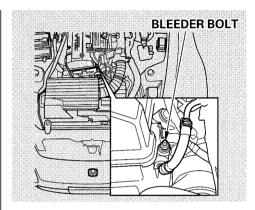
8. Loosen the bleeder bolt on top of the engine, and remove the bleeder cap near the engine oil fill cap. Pour coolant into the radiator up to the base of the filler neck. Tighten the bleeder bolt and reinstall the bleeder cap when coolant comes out in a steady stream with no bubbles.
