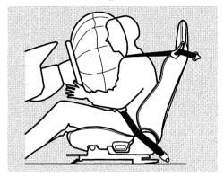
If you ever have a moderate to severe frontal collision, the sensors will detect rapid deceleration and signal the control unit to instantly inflate the airbags and activate the automatic seat belt tensioners.
