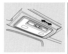
The interior light has a three-position switch. In the OFF position, the light does not come on. In the center position, the interior light comes on when you open either door. In the ON position, the interior light stays on continuously.
