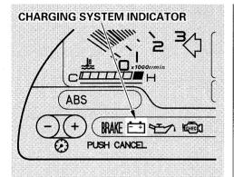
This indicator should come on when the ignition switch is ON (II), and go out after the engine starts. If it comes on brightly when the engine is running, it indicates that the charging system has stopped charging the battery.
