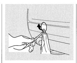
For very short distances, such as freeing the car, you can use the detachable towing hook that mounts on the anchors in the front and rear bumpers.
