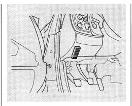
The interior fuse box is underneath the dashboard on the driver's side.
