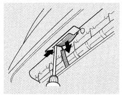
1. Insert a flat blade screwdriver between the left edge of the lens and the housing. The lens will come down.
