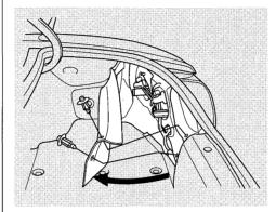
4. Determine which of the four bulbs is burned out: stop/taillight, backup light, turn signal, or side marker.
