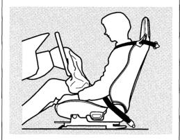
After inflating, the airbags immediately deflate, so they won't interfere with the driver's visibility, or the ability to steer or operate other controls.
