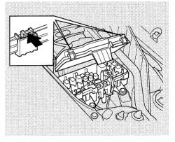
There are two under-hood fuse boxes in the engine compartment.
