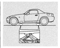
7. Locate the jacking point nearest the tire you need to change. It is pointed to by an arrow molded into the underside of the body. Place the jack under the jacking point. Turn the end bracket clockwise until the top of the jack contacts the jacking point. Make sure the jacking point tab is resting in the jack notch.
