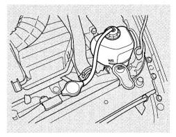
Look at the coolant level in the radiator reserve tank. Make sure it is between the MAX and MIN lines. If it is below the MIN line, see **Adding Engine Coolant** on page 161 for information on adding the proper coolant.
