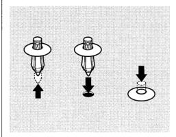
10.Install the trunk lining and secure it with the fasteners. To reinstall a fastener, reset the fastener by pushing on the pointed end until it pops back almost flush with the fingers on the housing. Put the fastener in the hole of the trunk lining and push on the center until it locks (the center is flush with the head).
