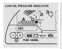
This indicator should light when the ignition switch is ON (II), and go out after the engine starts. It should never come on when the engine is running. If it starts flashing, it indicates that the oil pressure dropped very low for a moment, then recovered. If the indicator stavs on with the engine running, it shows that the engine has lost oil pressure and serious engine damage is possible. In either case, you should take immediate action.
