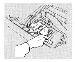
If the terminals are severely corroded, clean them with baking soda and water. Then use a wrench to loosen and remove the cables from the terminals. Always disconnect the negative (—) cable first and reconnect it last. Clean the battery terminals with a terminal cleaning tool or wire brush. Reconnect and tighten the cables, then coat the terminals with grease.
