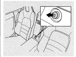
To use the accessory power socket, pull out on the cover. The ignition switch must be in ACCESSORY (I) or ON (II).
