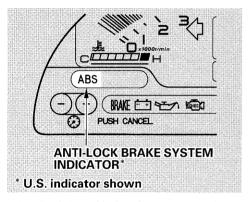
The ABS is self-checking. If anything goes wrong, the ABS indicator on the instrument panel comes on (see page 45). This means the anti-lock function of the braking system has shut down. The brakes still work like a conventional system without anti-lock, providing normal stopping ability. You should have the dealer inspect your car as soon as possible.
