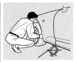
9. Remove the wheel nuts and flat. tire. Temporarily place the flat tire on the ground with the outside surface of the wheel facing up. Placing the wheel face down could mar its finish.
