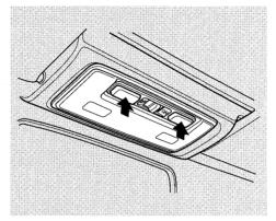
In addition, when the three position switch is in the center position with both doors closed, the two bulbs in the interior light can be turned on separately by the pushbutton switches next to them. Push the switch to turn the light on or off.
