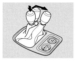
The 6-speed manual transmission has a lockout so you cannot accidentally shift from Fifth to Reverse instead of Sixth.
