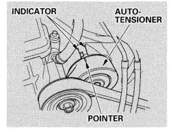
An auto-tensioner adjusts the tension of the drive belt.
