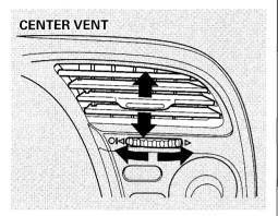
You can adjust the direction of the air coming from the vents on both sides of the instrument panel and at the corner of the dashboard on the passenger's side. To adjust the air flow up and down, move the tab in the center of each vent up and down. To adjust it left and right, turn the dial under each vent left and right.
