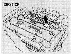
Check the engine oil level every time you fill the car with fuel. Wait a few minutes after turning the engine off before you check the oil.
