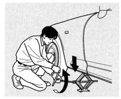
12.Lower the car to the ground and remove the jack.
