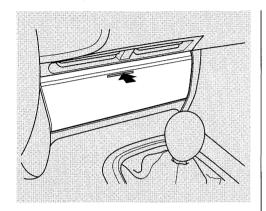
To open the audio panel, push on the top center and let the panel swing down. To close, pivot the panel up and push on it until it latches. Refer to page 94 for operation of the audio system.
