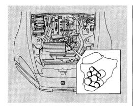
You should check the condition of the drive belt every 2 years. Examine the edges of belt for cracks or fraying.
