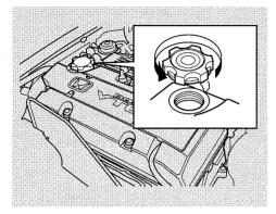
To add oil, unscrew and remove the engine oil fill cap on top of the left valve cover. Pour in the oil, and replace the engine oil fill cap.
