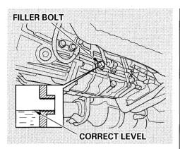
Check the fluid level with the transmission at normal operating temperature and the car sitting on level ground. Remove the transmission filler bolt and carefully feel inside the bolt hole with your finger. The fluid level should be up to the edge of the bolt hole. If it is not, add Genuine Honda Manual Transmission Fluid (MTF) until it starts to run out of the hole. Reinstall the filler bolt and tighten it securely.
