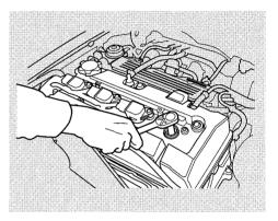
6. Torque the spark plug. (If you do not have a torque wrench, tighten the spark plug two-thirds of a turn after it contacts the cylinder head.) Tightening torque:
