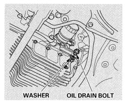
2. Remove the engine oil fill cap. Remove the oil drain bolt from the bottom of the engine. Drain the oil into an appropriate container.
