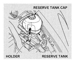
5. Remove the reserve tank from its holder by pulling it straight up. Drain the coolant, then put the tank back in its holder.
