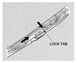
2. Disconnect the blade assembly from the wiper arm by pushing in the lock tab. Hold it in while you push the blade assembly toward the base of the arm.
