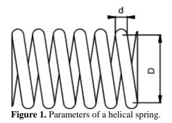
Since G is a constant, we wish to estimate  $S_{coil}$  by determining d, D, and N for each OE S2000 coil spring.
