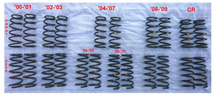
Figure 5. Photograph of the Honda S2000 OE coil spring components used for measurement.
